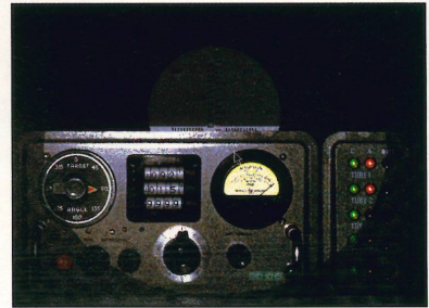
Loose lips don't sink ships, torpedoes do and this tatty little box programs the gyro-thingies in the torpedoes just to make sure. It all looks a bit primitive but this is 1940, remember.
